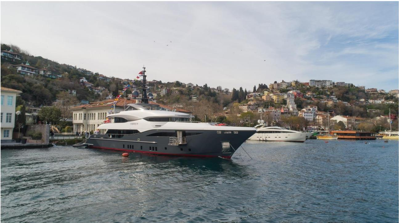
Starburst III is fitted with twin MTU 12V 2000 diesel engines, which gives her a top speed of 16 knots and a maximum range in excess of 4,000 nautical miles at 12-knot cruising speed. Launched in July 2017 and highly acclaimed ever after, the Bilgin Yacht 156 series continues with the new yacht 48m on spec Lilium which has a similar exterior look, but soft and minimalist lines in the interior. Lilium is planned to have debut in 2019 Monaco Yacht Show.
